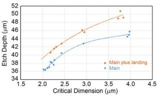
Figure 13: Depth after main etch (blue) and main plus landing etch (orange) versus trench width.
