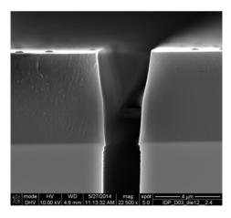
**Figure 10:** Detail view of the top of an etched trench with the photoresist still present.
