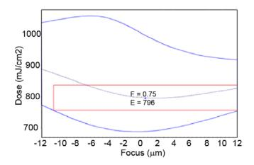
**Figure 8:** Experimental process window for  $2.64\mu m$  trenches. The blue curves indicate the  $\pm 10\%$  CD limits. The red box is the largest rectangular process window centered at the nominal CD. Sidewall angles are  $\geq 86^{\circ}$  as determined by cross sectional SEM.
