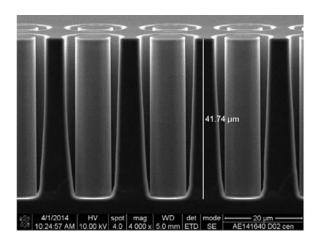
**Figure 5(b):** Cross-section of Donut TSV's etched in Si. The cleave is not perfectly perpendicular to the surface and it appears that the trenches are much narrower at the bottom which is not the case.
