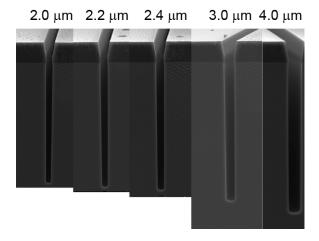
**Figure 9:** Cross-sections of etched trenches. The CD is of is labeled at the top of each trench. Note that the photoresist has not been removed.
