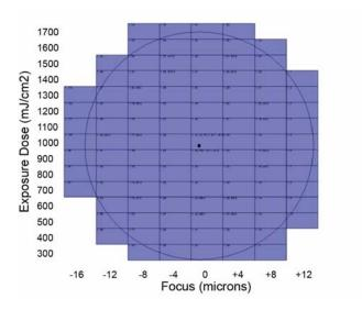
**Figure 4:** Wafer layout for the FEM. An eight by fifteen array was exposed with focus varying in the horizontal axis and exposure dose varying in the vertical axis.
