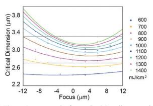
**Figure 6:** Bossung Plot for top CD 2.4μm linear trenches.
