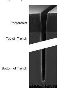
**Figure 11:** Cross-section of trench after main and landing etch. The landing etch at the bottom of the trench shows a smaller CD and more slope than the main etch at the top of the trench.
