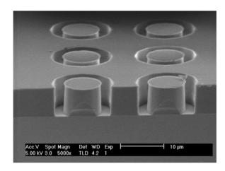
**Figure 5(a):** Cross-section of 2.4μm Donut TSV's imaged in 7.5μm thick positive photoresist.
