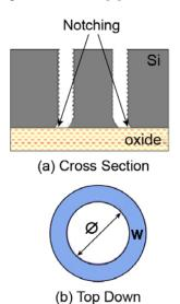
**Figure 2**: (a) Cross sectional drawing of the Si trench stopping on the STI oxide layer. (b) Top down drawing showing typical core width  $(\emptyset)$  and donut width  $(\mathbf{w})$ .
