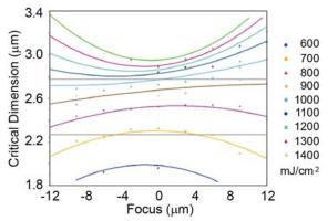
**Figure 7:** Bossung Plot for bottom 2.4µm linear trenches.
