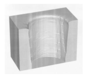
(a) Cross sectional contact with no defect.
