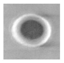
**3(c)** SEM of contact on wafer.
