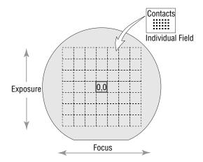
Figure 2: Wafer layout for exposure of the defect test reticle.
