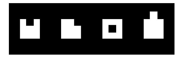
**Figure 1:** Illustration of the types of contact defects used in this study. From left to right are opaque edge center, opaque corner, opaque isolated center and clear edge extension defects.
