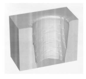
**(b)** Cross sectional contact with an opaque corner defect.
