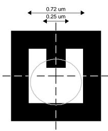
3(a) Layout of contact edge center defect with photoresist simulation contour.
