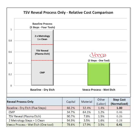
Figure 4. Direct TSV Reveal Process Step Comparison
