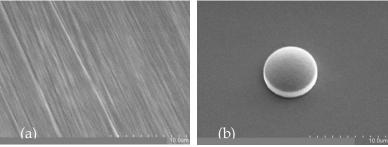
Figure 2. SEM images to illustrate surface roughness (a) Post Grind and smoothing (b) Post TSV reveal
