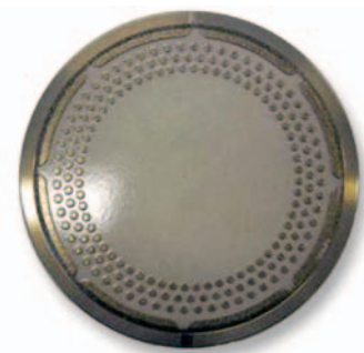
Figure 3. A prototype Mitsubishi Materials Corp. diamond conditioner disc coated with polytetrafluoroethylene.
